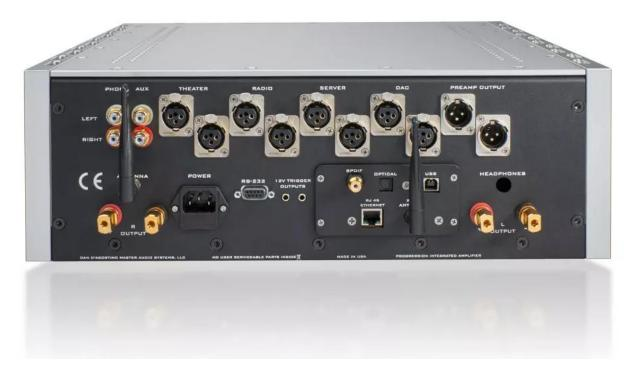
As for all the other inputs, every single one of them is balanced, in keeping with the amplifier's balanced circuitry (the output stage is also balanced). Rather oddly, rather than mounting the eight
